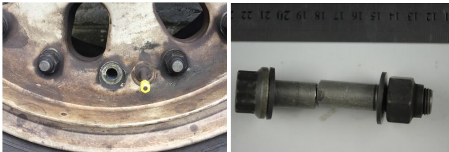
Figure 1: Macro appearance of installation site and broken bolt
